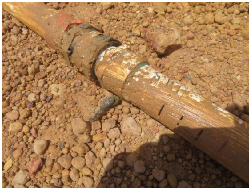
Figure 12. Close-up of a slotted PVC sample pipe immediately after extraction from the stockpile.
